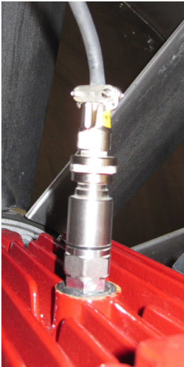
Sensor position on motor center (A1 : VTV 122)
