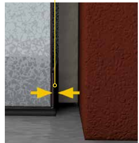
Strips of separation material
