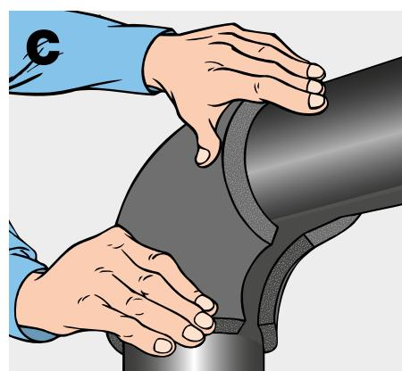
Bond the glued edges together by applying pressure.
