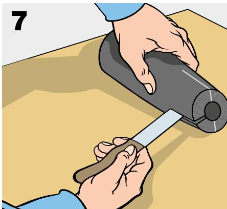
Glue the edges of the cut-outs together so that the diameter of the tubing reduces.
