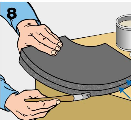
Allow the glue to dry and stick the edges together, starting from the two extremities.
