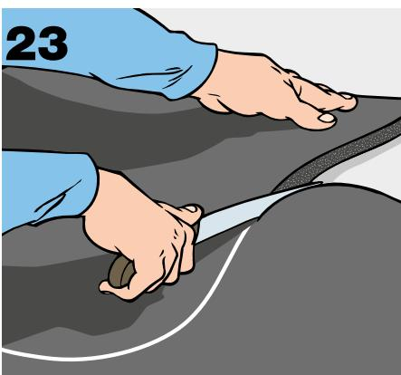
Chamfer the edges of the upper, convex curves towards the K-FLEX®'s inner surface.
