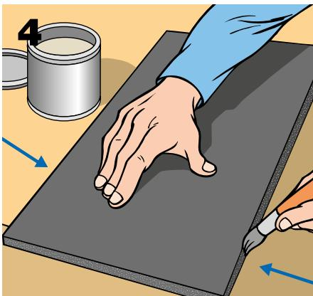
If the tubing thus created is not correctly lined up, push one against the other slipping the brush in the gap and twist until they are aligned.
